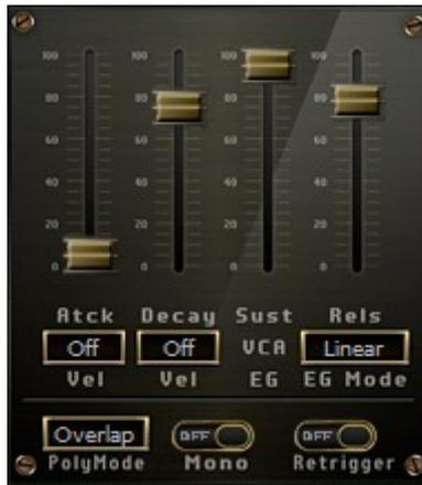
ADSR VCA EG for shaping the audiosignal in level, with three response modes: Linear, Exp(ponential), and Rev(erse) Exp(ponential) with the that being best for snappy envelopes. Attack and Decay can be lengthened or shortened by velocity.
