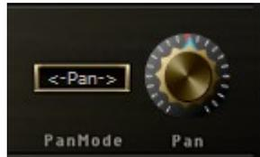
Pan has different modes as it controls both the undelayed and the delayed signal. Normal pan is to have undelayed and delayed signal move to left or right together. Next is to move delayed signal into opposite direction of undelayed signal. And some further modsources allow even more options for the delayed signal e.g. like Gator.
