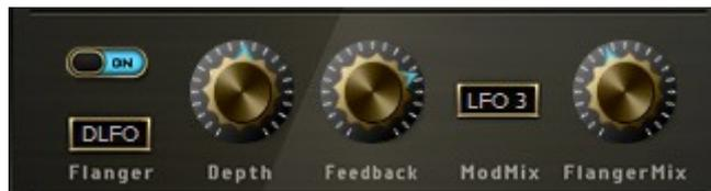
Stereo Flanger gives what you expect it for with basic controls for Depth, Feedback and Mix plus there are different modsources selectable for Depth and Mix. As there are two modulatable parameters you should try a manual setting for Depth and modulate Mix.
