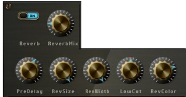
Stereo Reverb with basic controls for Width and Room/Size and Reverb Mix knob. In addition there is also a Low Cut knob to remove unwanted low rumbling frequencies in order to prevent the reverb from 'shattering'. You can even set a (short) predelay for the reverb to increase depth. Color is to have reverb more or less bright.
