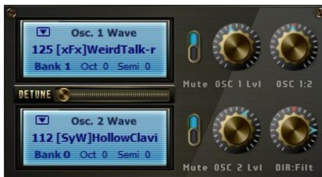
As sonic heart serve 2 pcm wave oscillators (using sf2 files with carefully selected waves). Each oscillator has options for semitone settings (0 to +11), octave (-2 to +2). Detune slider to spread both slightly off tune. Each oscillator has a Mute Button and a level knob for level adjustment. Both oscillators can be balanced to each other and this output can be balanced to direct out (of VCA) or the Filter.
