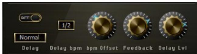
Though Delay is a mono delay it has dedicated pan option with modulations at the Pan Section, so you can really spread the sound in panorama. Delay is bpm synced in divisions of notelength plus settings and knob for manual offset. Knobs for Delay Level and feedback do what they are supposed to.
