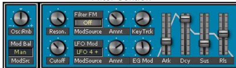
The section on the left is there to adjust the balance between the direct signal from the oscillators and the Rainbow section or modulat this. The output is valid for the filter section **and** Amplifier section's Direct signal input where it is balanced to the Filter output. Thus it is possible to have some interesting motions in the sound at this stage already.
