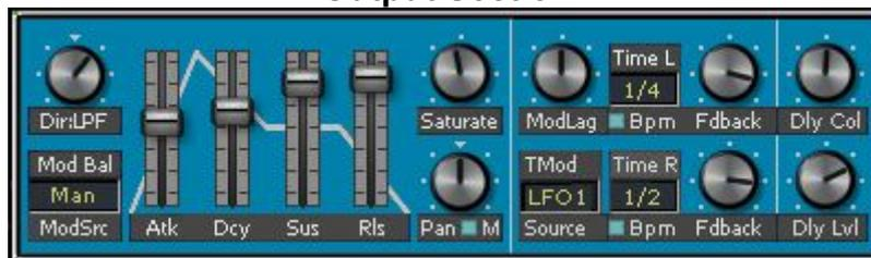
The input can be balanced bewteen the direct and filtered signal. The ADSR envelope generator determines the behaviour of the output level in time by Attack, Decay, Sustain and Release. Also an a saturation can be added to the signal and the pan position adjusted or modulated by selected LFO 1 to LFO 4.
