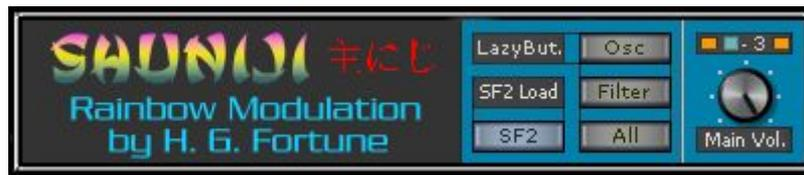
The Lazy buttons allow random changes of selected parameterd separate for oscillator-, filter- and all sections (All).
