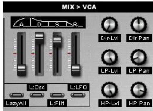
The output section provides an [ **A** ] [ **D** ] [ **S** ] [ **R** ] envelope generator for shaping the overall signal with **A**ttack, **D**ecay, **S**ustain and **R**elease. Also You can mix the amount of level from outputs of direct(unfiltered signal), Lowpass and HiPass filter. In addition to this there is an independant pan-setting for each output.
