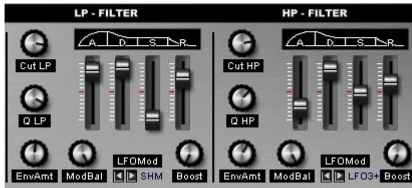
There are two independant filters one 24dB lowpass filter with resonance **[Q]** and a 12dB hipass filter with resonance. Each filter can be modulated by an ADSR-EG and/or a selectable modsources from the LFO-section. The **[ModBal]** determines the amount of modulation between ADSR EG and LFO-source. The **[Boost]** knob provides an adjustable enhancement of the current filter frequency.
