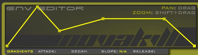
The two envelopes in this instrument are slightly different. The **VCA Envelope** is a straightforward **ADSR** jobbie, whilst the **Modulation Envelope** has an extra segment before the Sustain level is reached.
