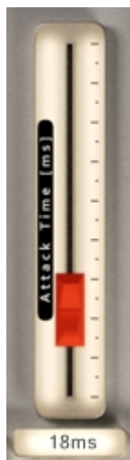
Figure 13: Attack slider set to 18 milliseconds
